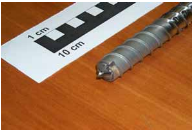
Corer (drilling and coring configuration, collected sample)
