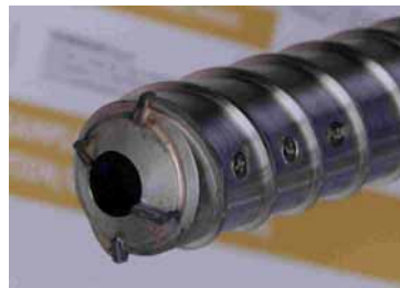
Drill rod with shutters (drilling and coring configuration, collected sample)
