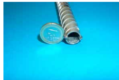
Corer (drilling and coring configuration, collected sample)
